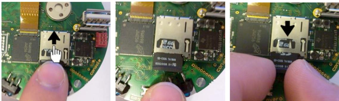
Once the card is removed, it's possible to read and write its content on a computer through the USB adapter. In order to re-insert the micro SD, insert it in its place and push it again:
