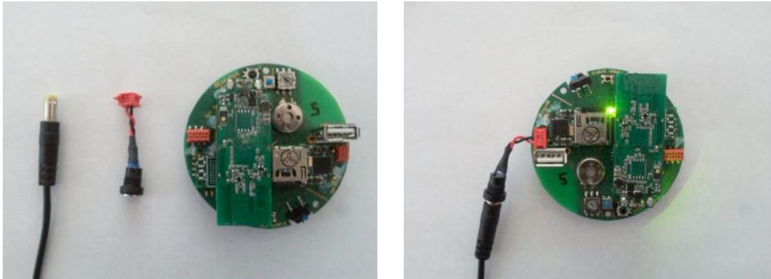
You need to simply attach the power supply in one side, and the other side of the external power cable on top of the extension (near the USB plug). Once the cable is connected a green led should turn on indicating that the extension is running, as shown in the previous figure (right).
