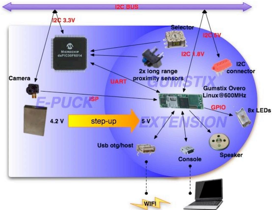
The following figure illustrates where the components are physically placed on the e-puck extension board for the Gumstix Overo COM.
