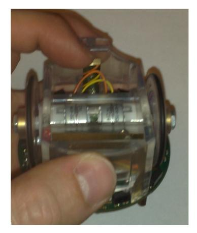
Now you can bend the upper side of the contact in order to make easier the contact with the battery:
