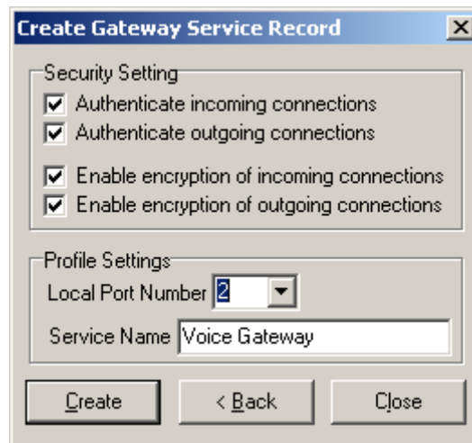
Figure 4-26. Configuring the profile settings for HSAG
