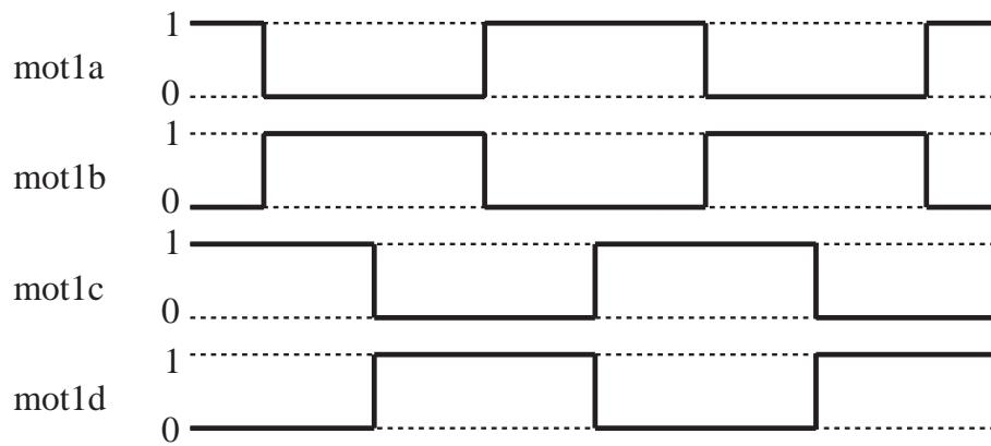
Figure 17: Activation sequence for the motor 1 control signals.
