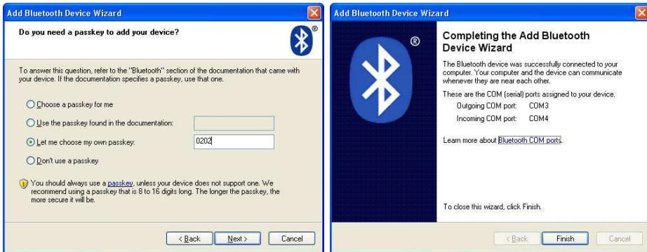
Figure 14: Enter the pin code corresponding to the number of your e-puck robot. The wizard will set a COM port corresponding to your robot.
